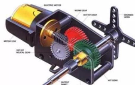
Construction of Servo Motor
