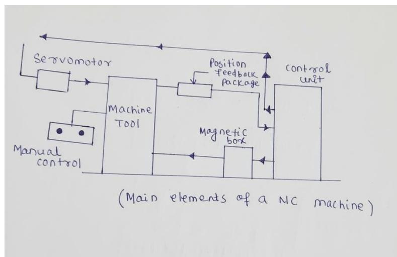
The main elements of a NC machine tool are :-
