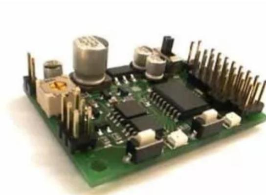
Think of the controller as the brain of a robot. It is the central operating system that controls how all other parts of the robot work. It is programmed with software that enables it to receive, interpret and execute commands. In more advanced robots, the controller can also have a 'memory' from which it executes repetitive tasks as it 'remembers' how they work. Artificial intelligence in smart robots is also inbuilt into the controller via software.
