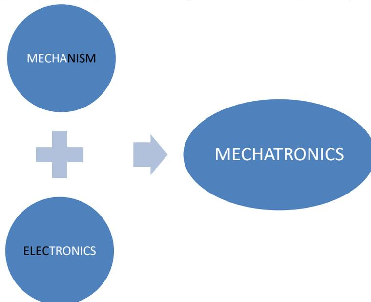
Mechatronics brings together areas of technology involving sensors and measurement systems ,drive and actuation systems , and microprocessor systems , together with the analysis of the behaviour of systems and control systems .
